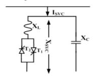
Figure 1. Equivalent circuit of SVC
