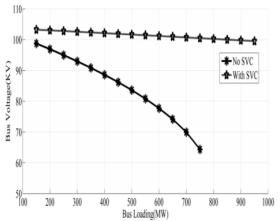
Figure 6. Bus voltage's diagram under different loading
