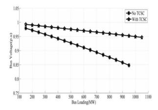
Figure 8. Bus voltage's diagram under different loading
