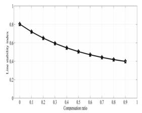
Figure 5. VCPI's diagram with compensation by SVC
